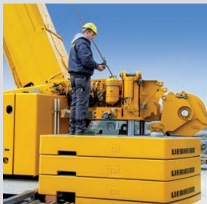
Self-mounting of ballast and optional hoist gear 2
